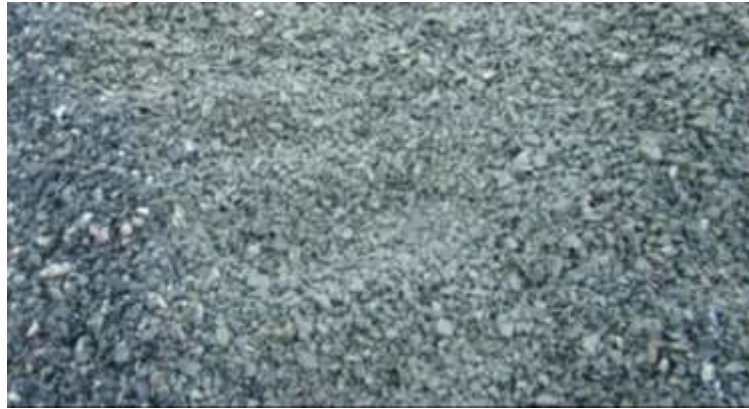
Figure 3.1. Typical Angular \frac{3}{4} " Stemming Material
