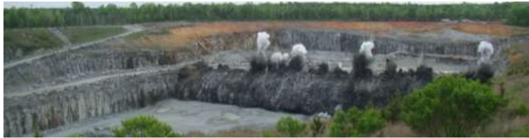
Figure 4.9. Shot 1 Stemming Ejection
